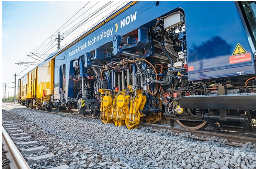
Track tamping machine Plasser & Theurer (©Plasser & Theurer, 2022)
